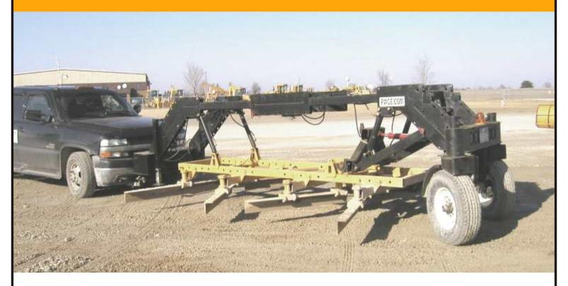
This attachment is limited only by the end user's imagination. There is any number of possibilities for this attachment. Any category of 3-point hitch attachments or skid steer quick coupler attachments can be used with the Construction-Carry-All (CCA). This system allows the operator to hook up various attachments and switch drive units with little effort.
