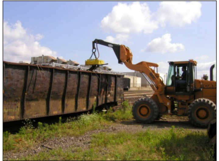
The PWCE JIB MAGNET is a 8 foot jib with a large 36" magnet attached.
