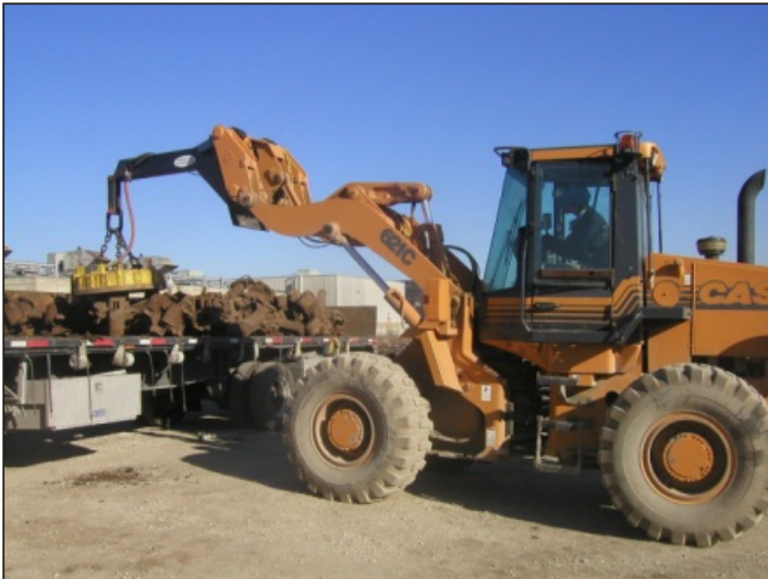
The PWCE JIB MAGNET is a 8 foot jib with a large 36" magnet attached.
